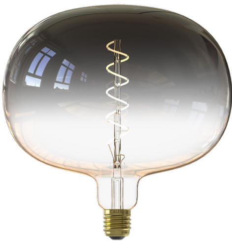
Boden Gris Art. # 426278 EAN 8712879147534 1800K, 5W, 130 Lumen Dimmable Ø: 220mm, H:225mm
