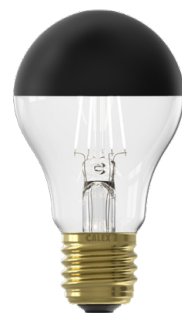
Standard A60 Top Mirror Black Art. # 20 01 0002 00 EAN 8712879150695 1800K, 4W, 180 Lumen Dimmable Ø: 60mm, H:105mm
