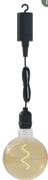
Outdoor Battery Terlizzi Pendant Light Art. # 43 01 0026 00 EAN 8712879162001 1W, 2200K, 4 Lumen, IP44 incl. remote controle 4 x AA, batteries not included cable lenght 1,2m
